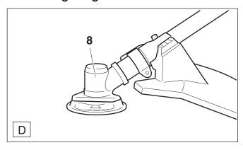
After about 50 operating hours the gear box (D/8) should be checked by a OLMAR service centre, and if necessary regrease.
